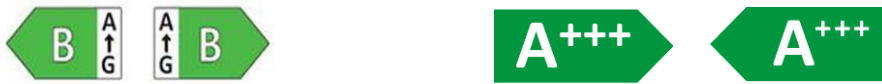
Figure 1. Graphic arrow for nested displays of the energy label; on the left for products that received the new generation of energy labels and on the right those that have not yet received the new energy label.
